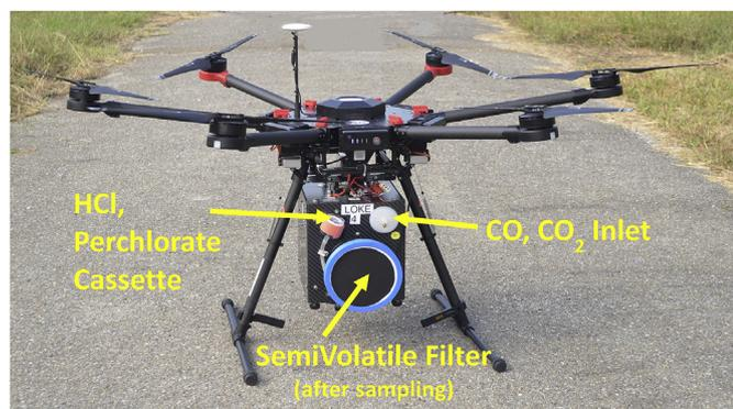
Fig. 1. UAV with attached lightweight instrument sampler, Kolibri – Loke version.
