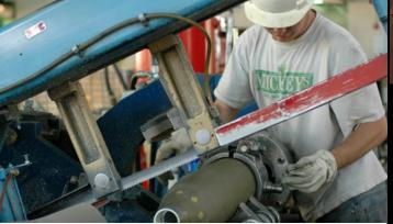
Recovery, reuse, and recycling processes disable and decontaminate surplus, obsolete, and inoperable munitions using various methods of disassembly, size reduction, and explosives decontamination.
